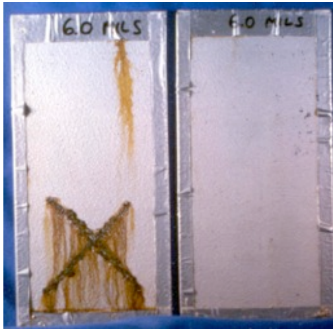
2500 hrs. salt fog U-104 over pre-rusted panels
