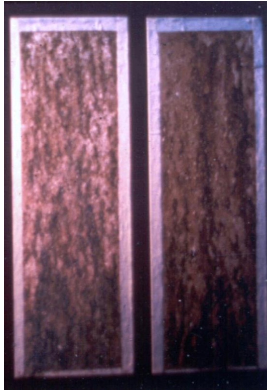
Three-Coats Alkyd On Pre-Rusted Panel After 1,024 hrs in Salt Fog
