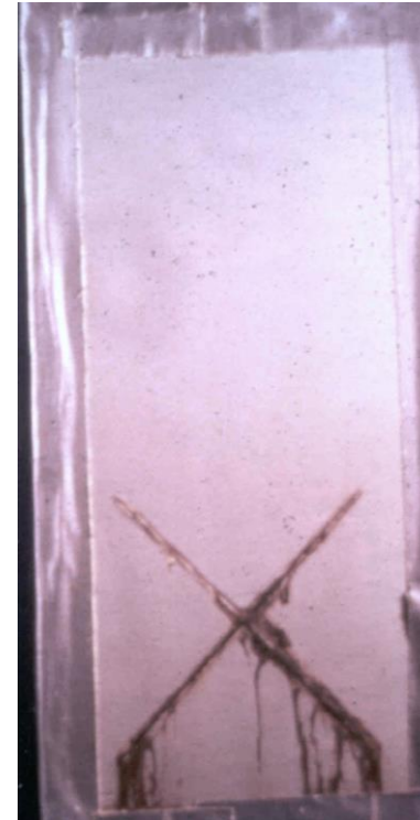
14,000 Hours Over Pre-Blasted Panel Demonstrates Minimal Undercutting
