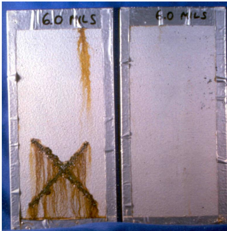
Typical ASTM B-117 Test at 2,500 Hours. U-104 Over Pre-Rusted Panels
